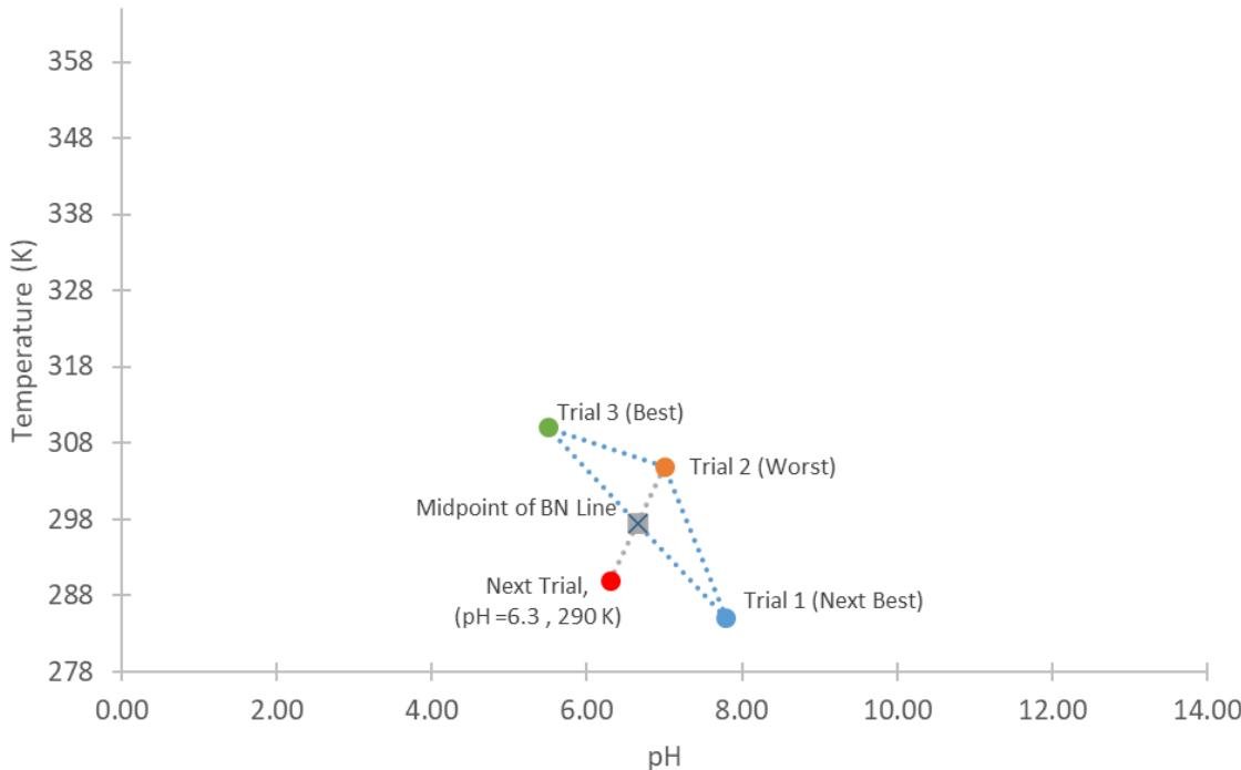
Above is a depiction of what a Simplex method might look like for the first three measurements and the prediction of the next measurement. What is shown is **not** a complete experiment, this is only the start of the process to demonstrate how the next set of conditions would be selected.
